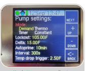
Use buttons corresponding to icons to cycle current selection in red. Use "DOWN" or "UP" buttons to increase or decrease temps and times
