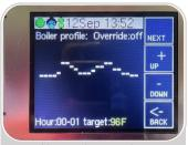
This page shows a 24 hour schedule, each line represents one hour of the day which is indicated at the bottom. Change each hour to desired lock out temp. Use "NEXT" button to advance to the next hour, use "UP" or "DOWN" to increase or decrease temp.
