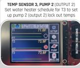
Press **"BOILER"** button to advance to boiler settings
