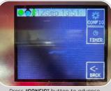
Press **"CONFIG"** button to advance to pump settings Press **"TIMER"** to set up off times
